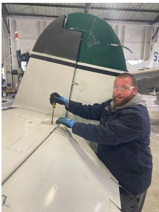
Jason Beaver changes a bonding strap on the C45 during annual maintenance and safety standdown.
