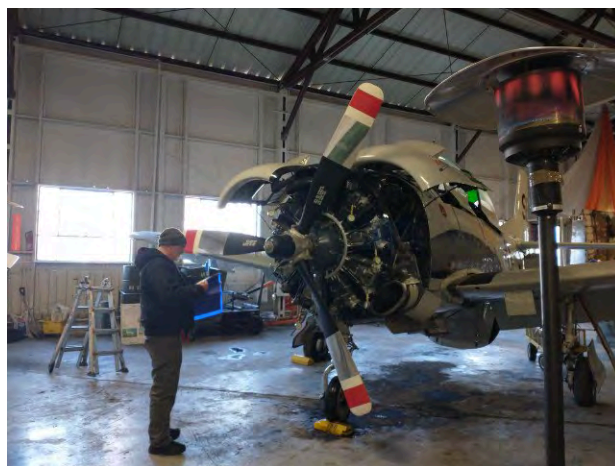
Frank Fry performs the compression test on the T-28 B.
